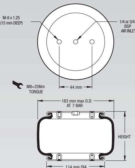
**NOTE:** A bead plate part is shown. This part is also available with bead rings. Bolts are not included. See pages 8-10 for explanation.
